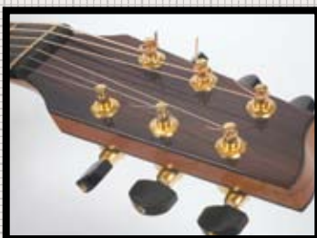
■ The headstock is set at a steeper angle to increase string tension for lowered tunings
